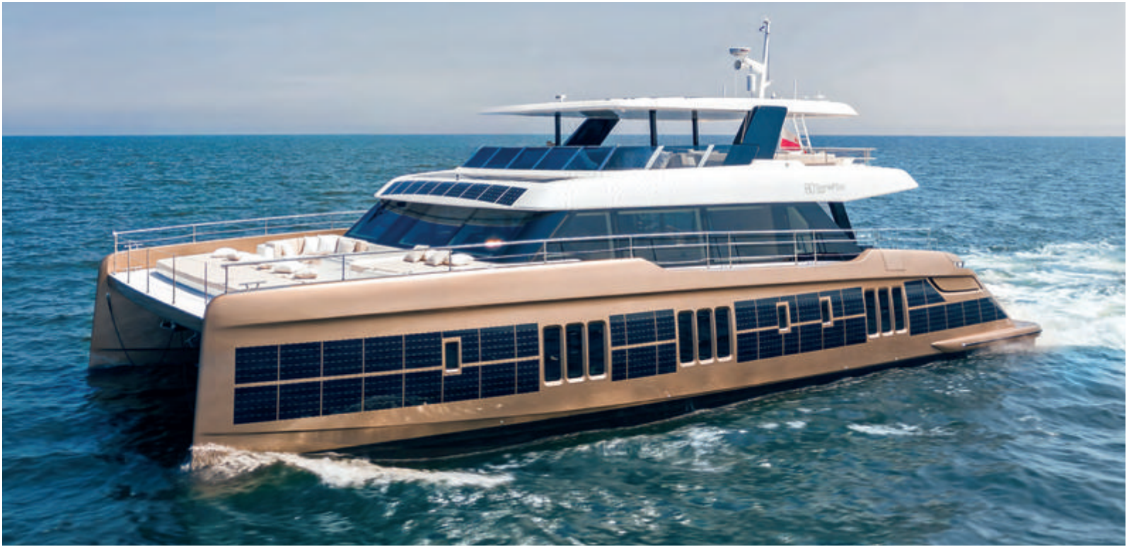
An 80 Sunreef Power Eco, Sol features the Polish yard's revolutionary solar panels integrated into the hull sides and superstructure
