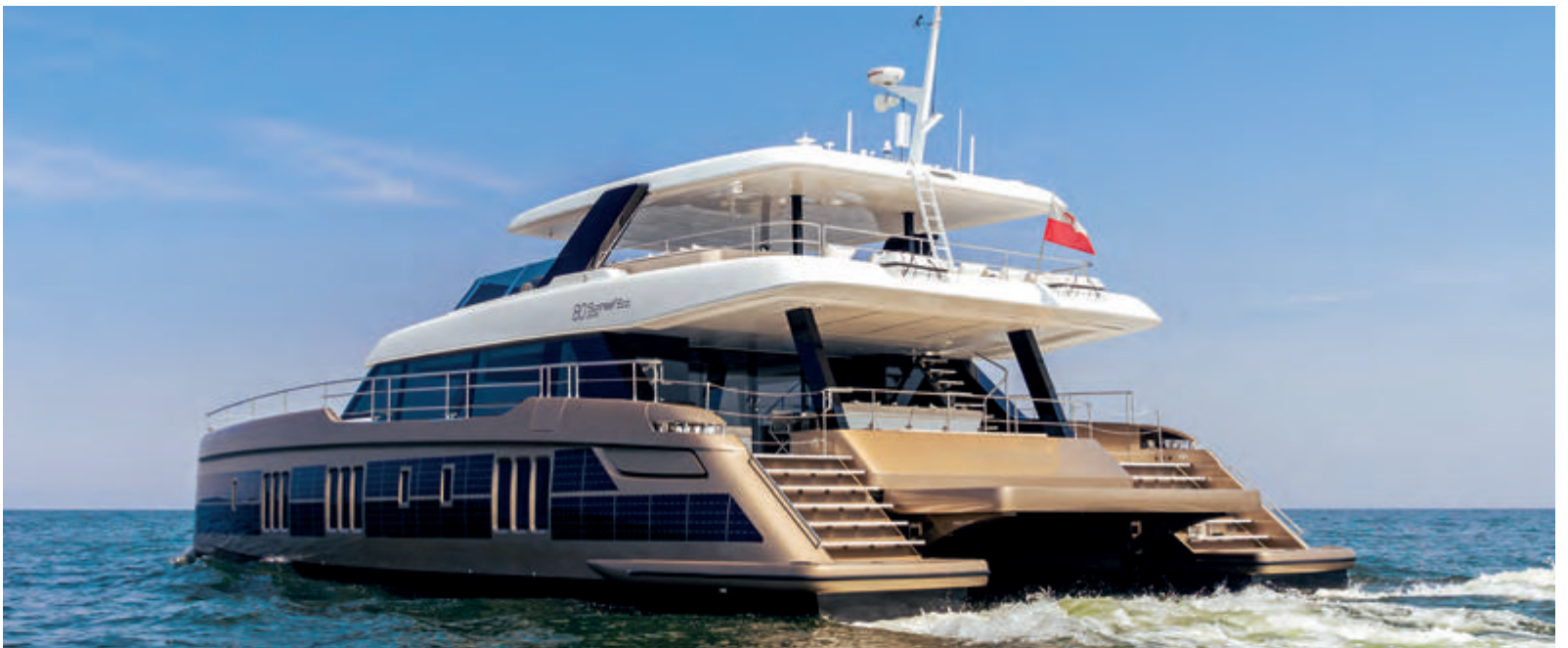
Sol has two 360kW electric engines, 990kWh of batteries, an energy-saving air-conditioning system and smart energy management
